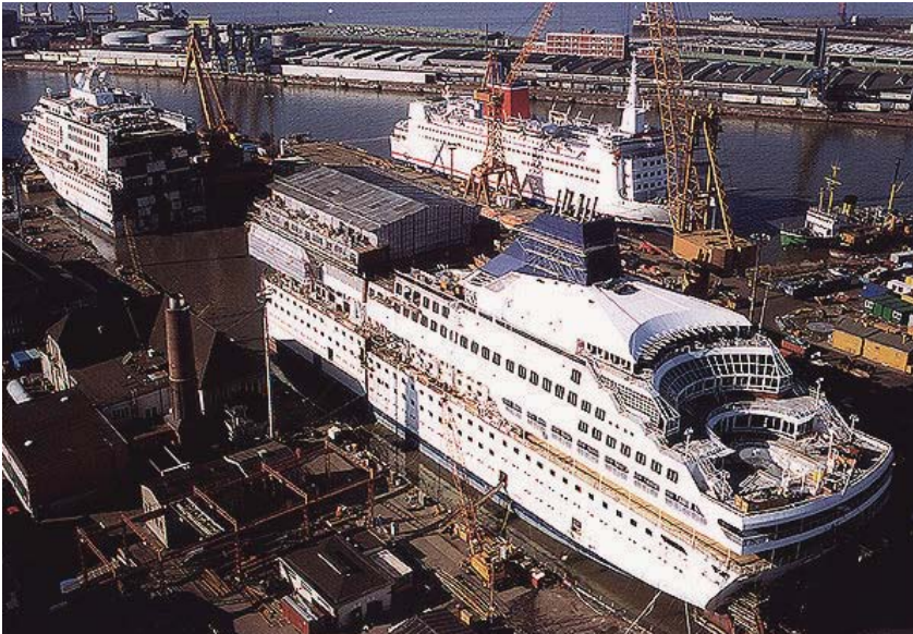
"Stretching" a ship in 60 days: Norwegian Dream undergoes lengthening
